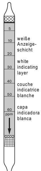
**NL - Zwavelwaterstof 5/b (CH 29 801) Dräger Tube®**
